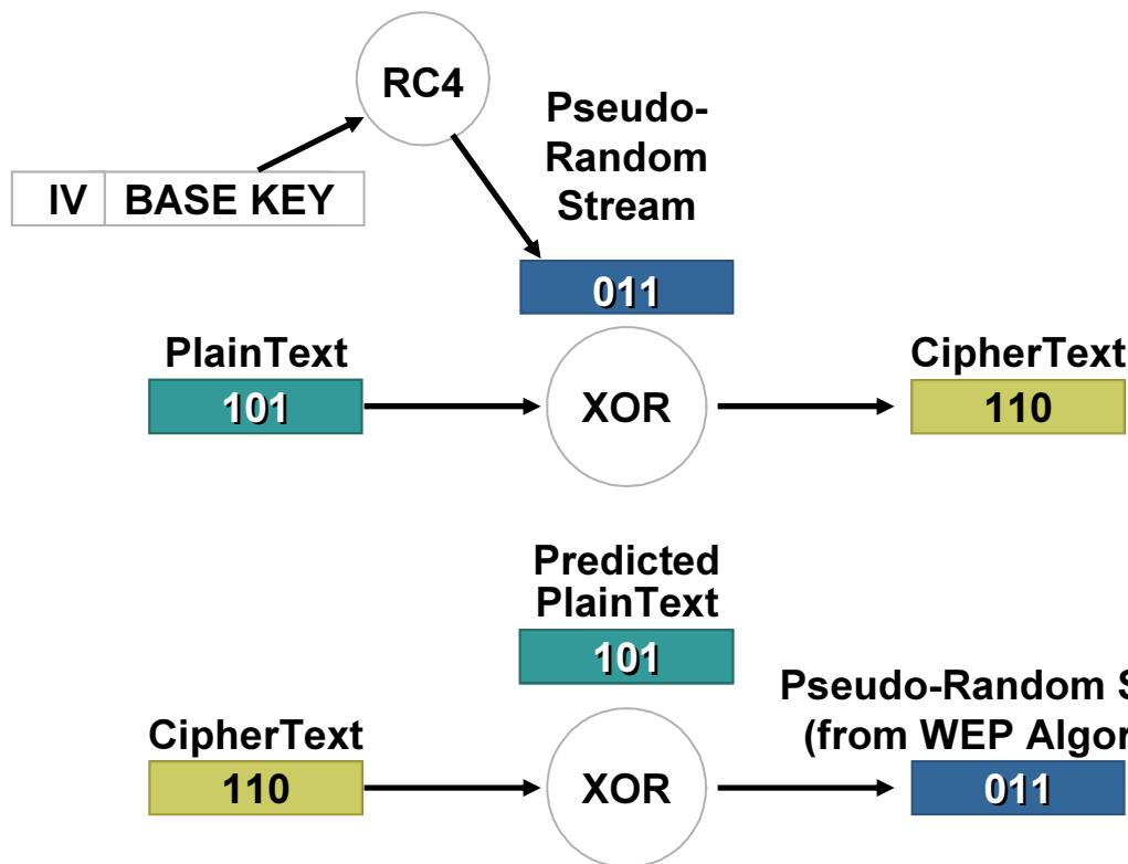
**Encryption:** The Pseudo-Random Output from WEPs RC4 Cipher Is XQRed with the Plaintext Data to Produce the Ciphertext
