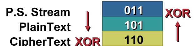
**Known Plaintext Attack:** If Ciphertext Is XQRed with Known (or Guessed) Plaintext, the Stream Cipher Output Can Be Derived
